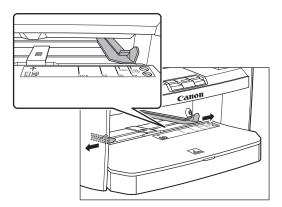
When setting paper, gently insert the paper into the multi-purpose tray with the print side up.
